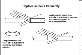
Screens should be replaced whenever the hammermill capacity decreases or product quality begins to deteriorate. A drop of 15-20% in capacity is a good indicator that the screens should be replaced. Replacement screens should have an equal percentage of open area as new screens and the screen hole stagger should correct. Low cost screens will often have less open area (more space between the holes) and can reduce hammermill capacity by 20-40%.
